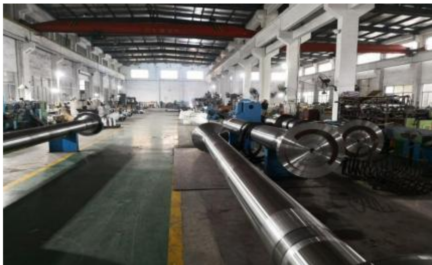
Marine shafts (propeller shaft, intermediate shaft, rudder stock, rudder pin)
